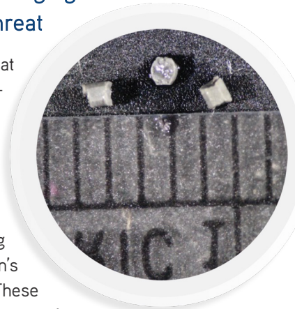
Less than 5mm long, microplastics easily pass through water filtration systems into rivers, lakes and oceans.
